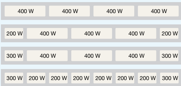
Fig. 79: Four examples of radiator equipment for an EBF/100 construction element
